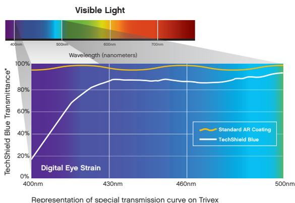
Figure 6. Spectral transmission of TechShield Blue.
