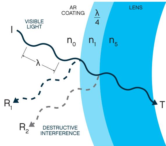
Figure 2. How an AR coating creates destructive interference Illustration: <https://commons.wikimedia.org/wiki/File:Optical-coating-2.png>
