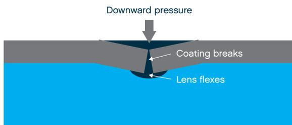
Figure 4. Scratch formation on an early AR-coated lens.
